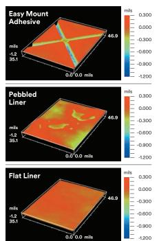
Microscopic view of adhesive surface measured with interferometer.
