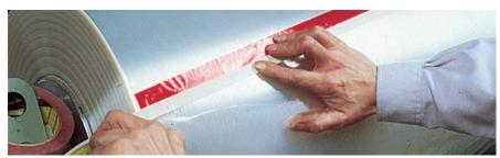
With high tack and good shear strength, 3M™ Double Coated Tape 9420 splices plastic film quickly and securely. Red carrier identifies the splice for later removal.
