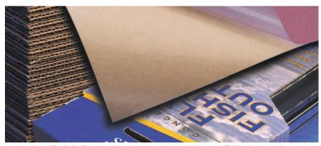
Designed specifically for flexographic printing on corrugated board, 3M<sup>™</sup> Thin Flexographic Mounting Tape 2205 is a 5-mil double-coated polyester film tape with cross-hatched adhesive. The cross hatching reduces air entrapment, saving time and improving print quality.
