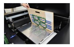
**3. Main Unit (press unit)** The main press unit uses patented moving press rollers to press the paper. This makes the die cutting process much quieter and more power efficient than conventional die cutters.
